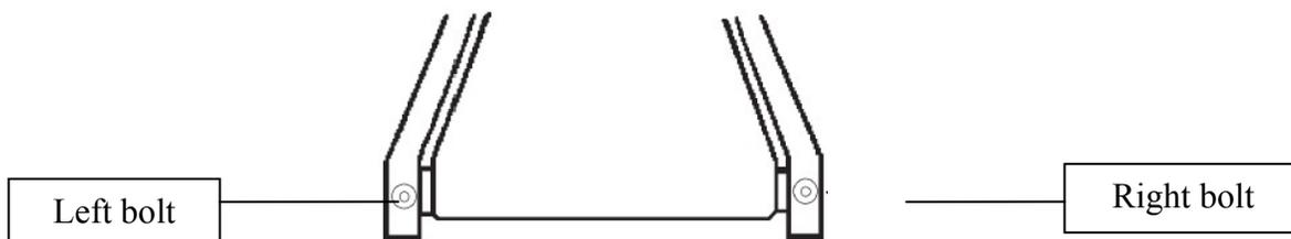
**Note: Adjustment is thru the small hold on the end caps.**
